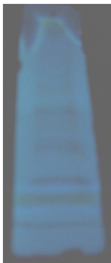
Figure (2): the TLC plate showing separation of Castor leaf ethyl acetate extract under UV
