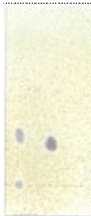
Fig. 2: Silica gel thin layer chromatography for Quercus infectoria with standard Gallic acid
